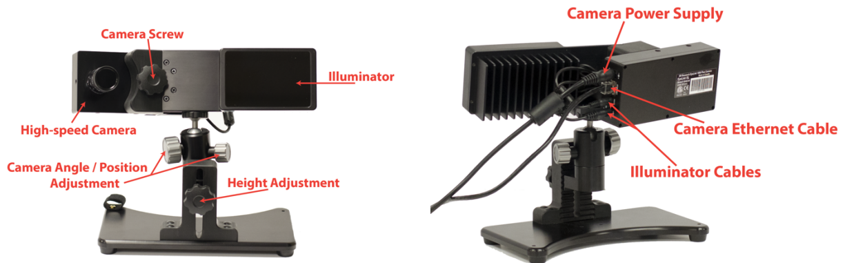
Figure 3-2: Parts of the EyeLink 1000 Plus Desktop Mount
